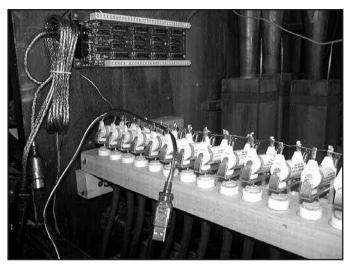
Figure 10. The MIDI circuit board is mounted on the left side of the case. The USB cable connects the Yamaha interface to the computer.
