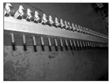
Figure 1. Manifold board with Peterson valves on top and  $\frac{1}{4}$ " copper tubes below each one.
